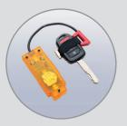
Data detection. When indicated by the cloning device, wrap the U-Snoop around the customer key and turn the key in the car ignition 2 times. U-Snoop LEDs illuminate to confirm successful sniffing.
